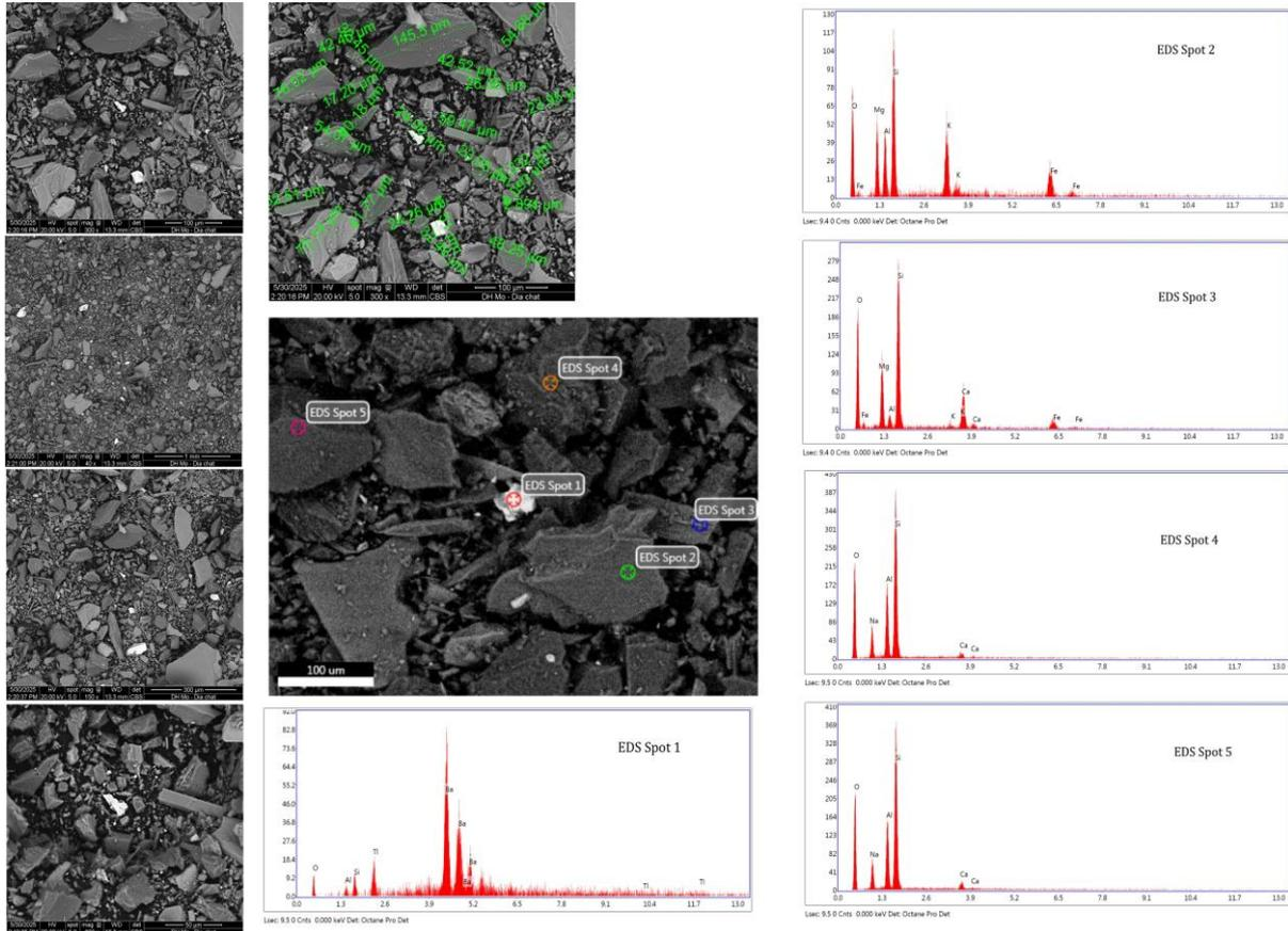
Figure 2. Images of tailing sample using SEM-EDS.
