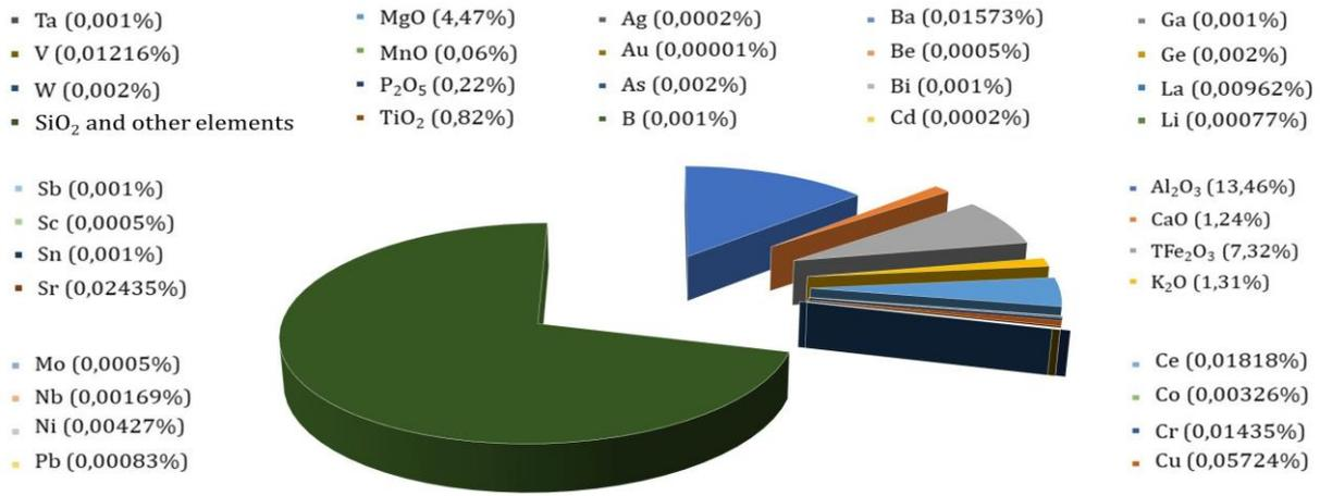
Figure 5. Chemical composition of tailing using ICP-MS.
