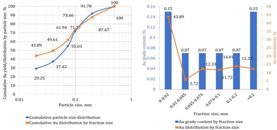
Figure 1. Particle size distribution of the Ta-Phoi cooper tailing.
