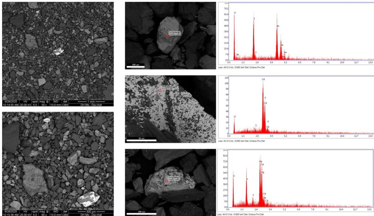
Figure 4. SEM - EDS images of the tailing sample after Au upgrading by shaking table.
